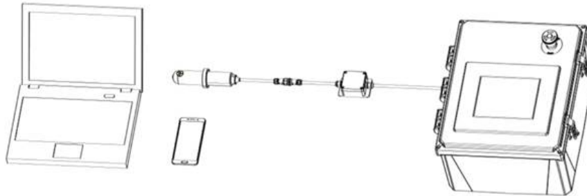
Figure 4. Bluetooth connection to ST-588 probe
